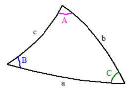
Spherical trigonometry shows that to compute all the values of a spherical triangle, we must know any three of the six sides or angles; this results in 20 cases. By permutation, we can reduce this number to 6 cases. Finally spherical trigonometry establishes, with the aid of the so-called polar triangle, a duality between the sides and angles, which allows us to divide this number by 2. The result is that, to solve a spherical triangle, we must know how to treat the following 3 cases:
